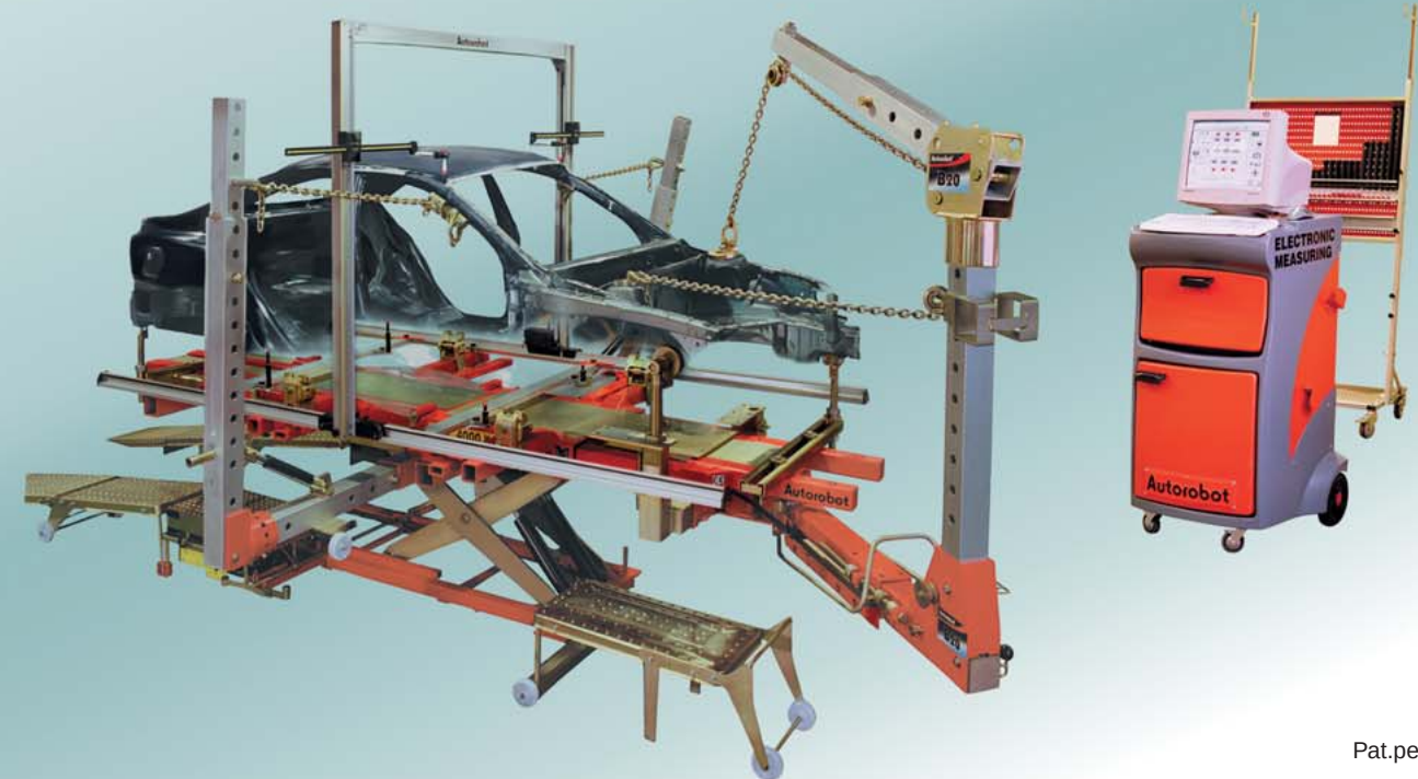
The picture shows B20 Gold set and mechanical/electronic measuring system
